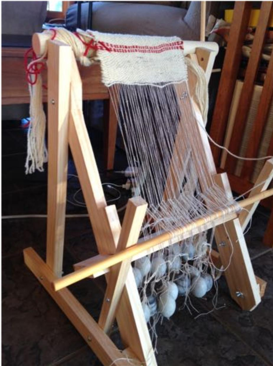
Figure 11. The finished loom with warp and weaving installed.
