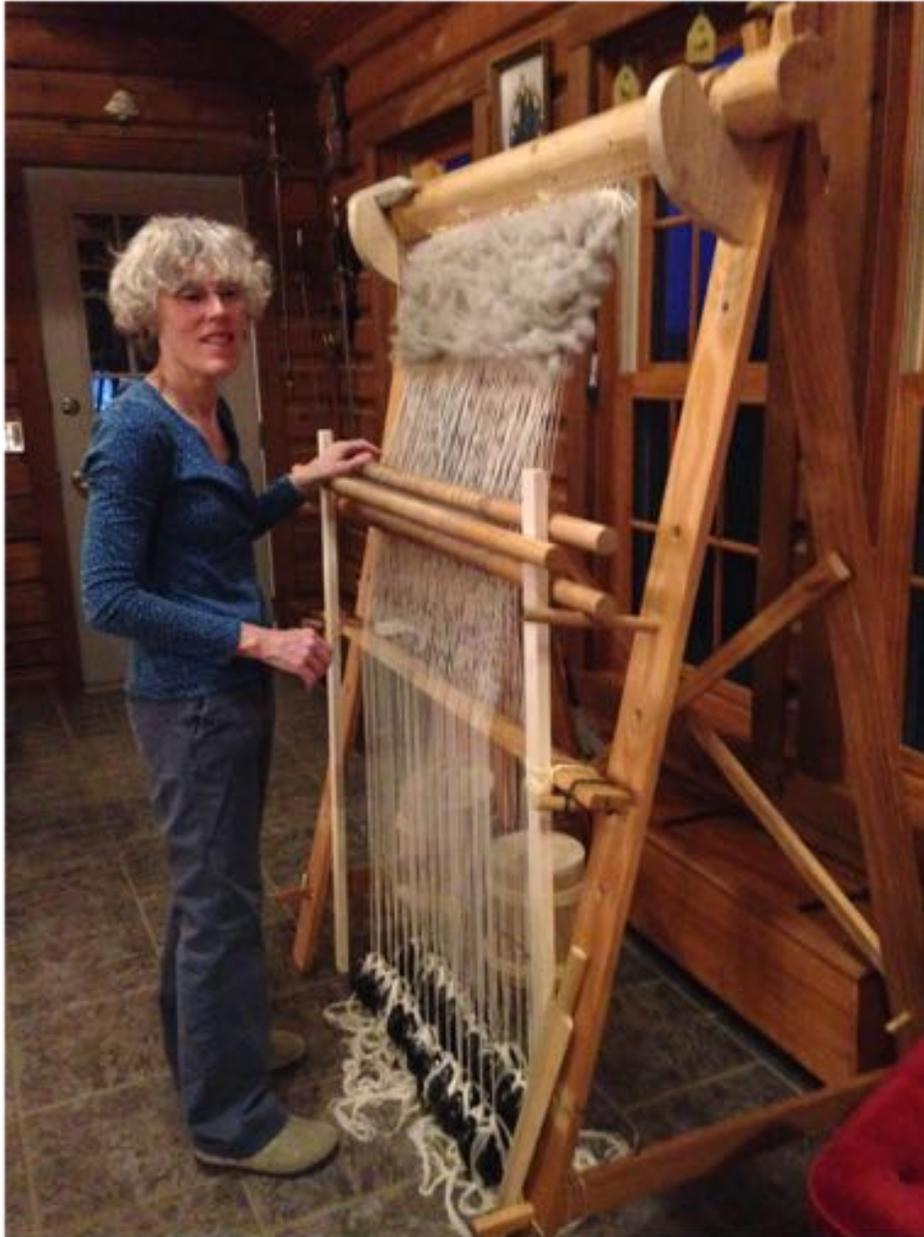
Figure 1. A Warp-Weighted loom configured like those of Iceland for rya on 2/2 twill. This loom is portable, and fashioned after those used in classes at the Vesterheim museum.
