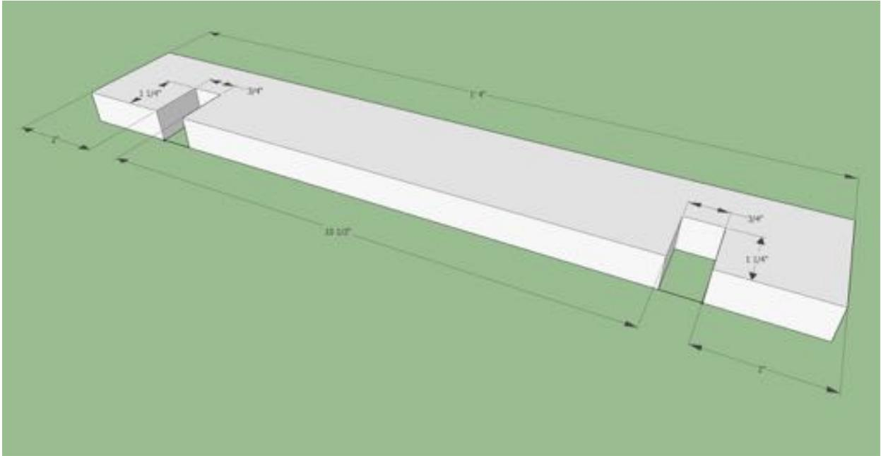
Figure 7. The cross piece and shed rod.
