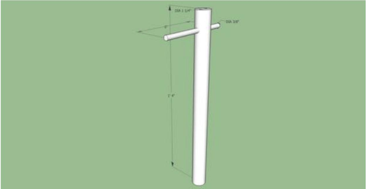
Figure 10. Warp beam with roller rod.
