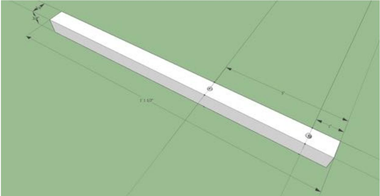
Figure 9. The vertical heddle support rod.
